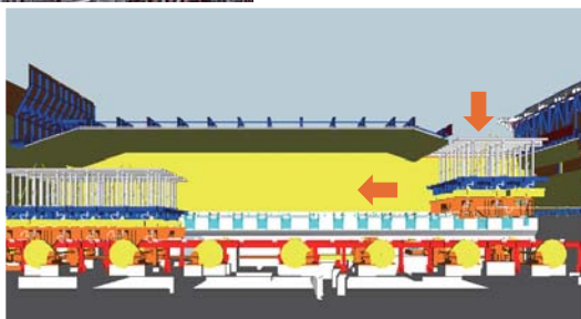
▶ Drive unit modules inserted in sequence from the ceiling hatch of the furnace
