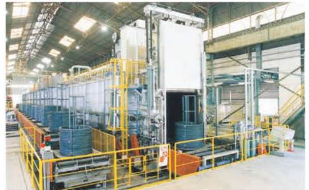
Roller Hearth Type Wire Rod Coil Continuous Annealing Furnace 辊底式线材卷连续退火炉
