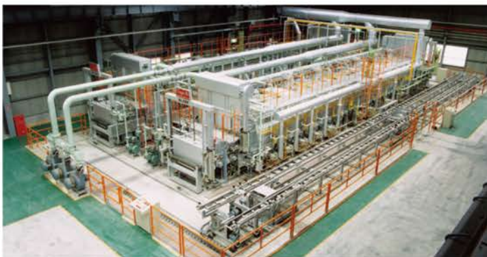
Continuous Deoxidization Annealing Furnace 连续无氧化退火炉
